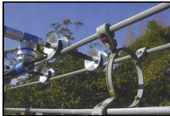
Figure 10. Expliner Overcomes Cable Spacers of Different Shapes and Sizes [19]
